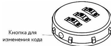
In order to change the lock code, you need to press the button on the lock and, while holding it, to change the digital code to the required one.
